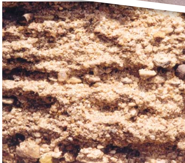
Right: Close-up of gravel and coarse sand-sized material from the Ogallala Formation. (OGS photo).
