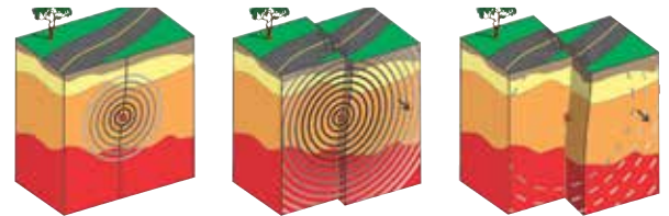
Figure 1 Figure illustrates how a fault might look and how buildings and roads on the fault are damaged when a fault slips and an earthquake occurs. The black rings represent the seismic energy as it radiates away from the epicenter. As the amplitude of the wave decreases it goes to gray. Modified from the USGS.
